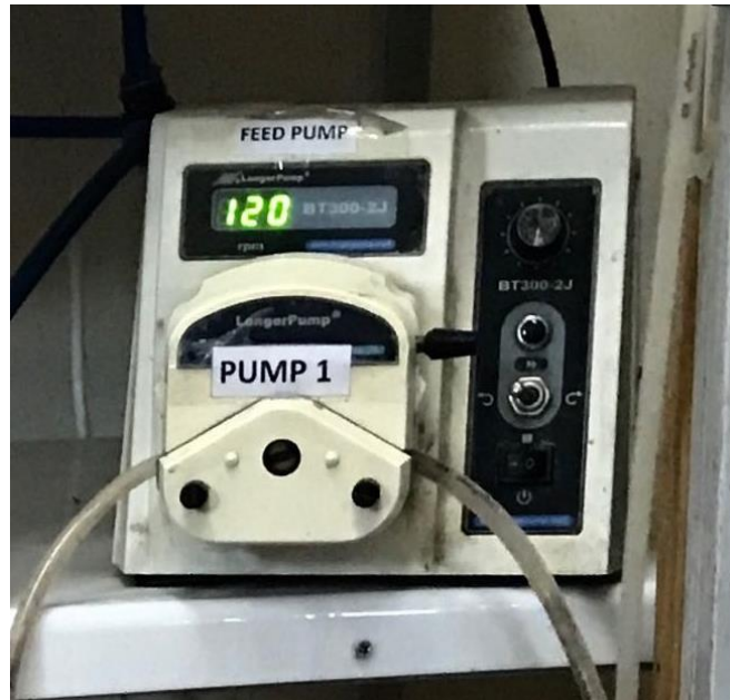
Figure 3.6: Pump that was used in the continuous system
