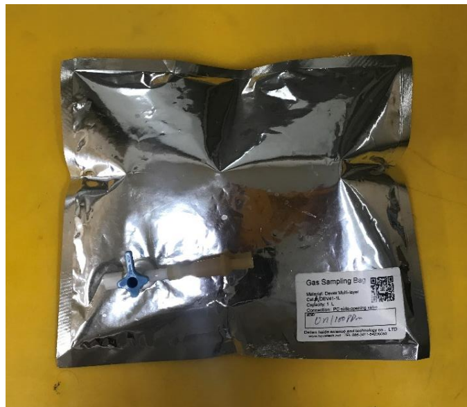
Figure 3.5: Gas sampling bag was used to collect the hydrogen gas produced from electrocoagulation
