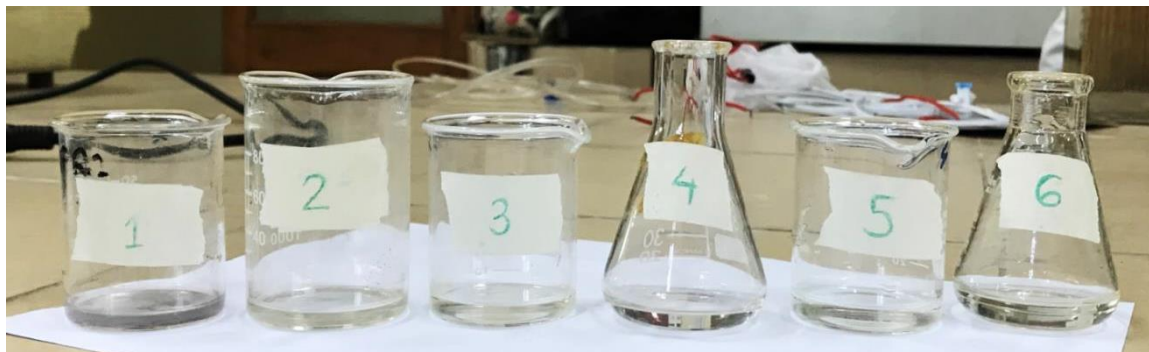
Figure 4.6: Samples drawn at different time intervals from the batch system at 12V, pH 8 and room temperature
