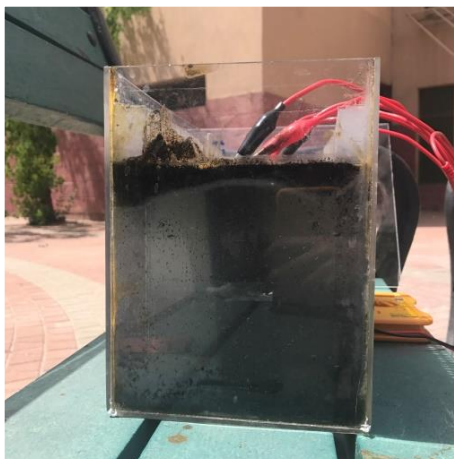
Figure 4.10: Final color of the wastewater sample after electrocoagulation
