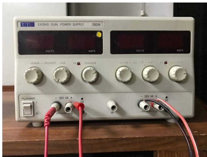
Figure 3.2: Power supply that was used to provide voltage to the electrodes
