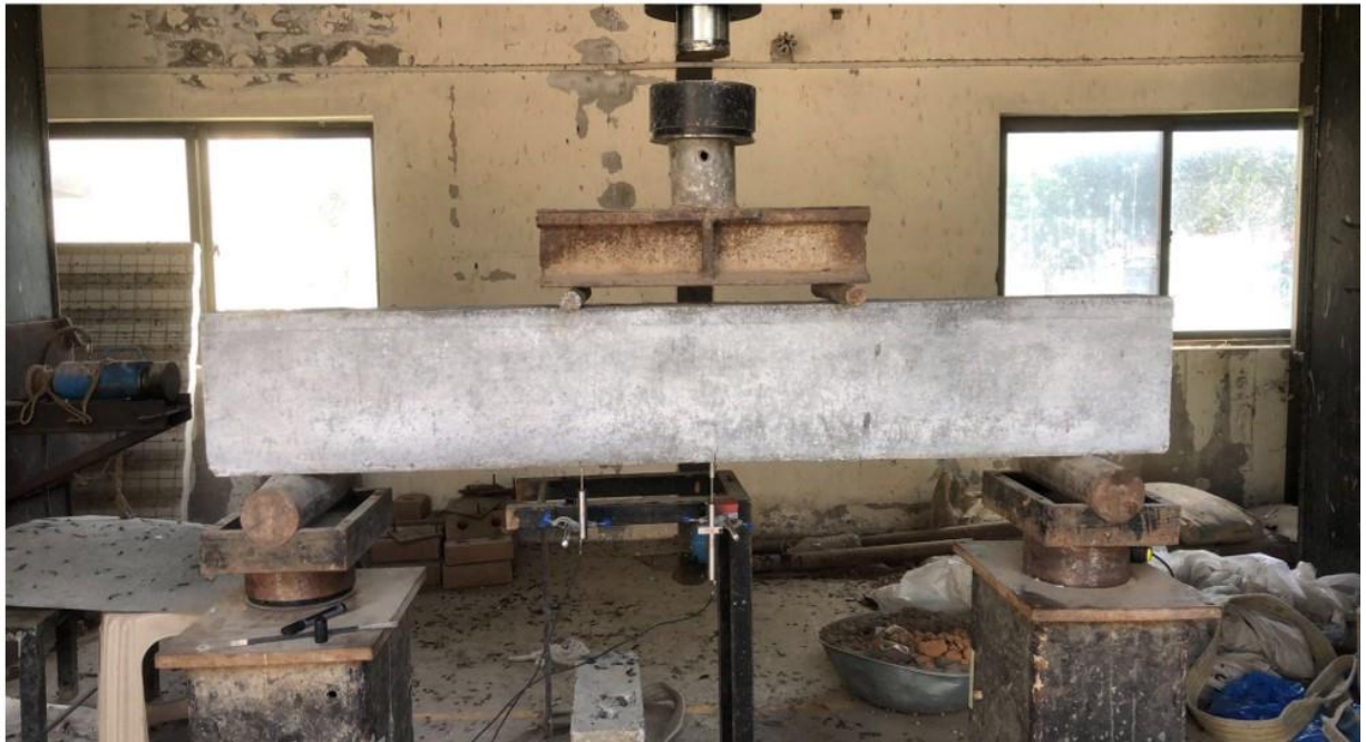
Fig. 6 feet beam testing
