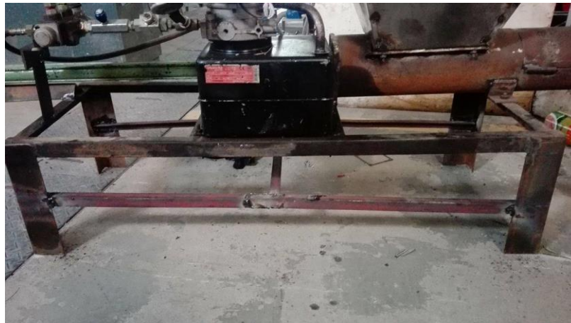
Figure 8: Welded angled irons
