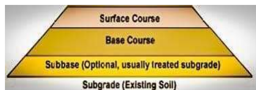
Figure 2.1 Typical conventional pavement cross section
