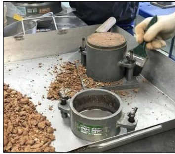
Figure 3.2: Proctor Apparatus taken after Timely Engineering Soil Tests, 2010
