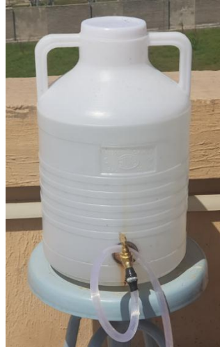
Figure 3.12 Feed water tank with tap to control flow
