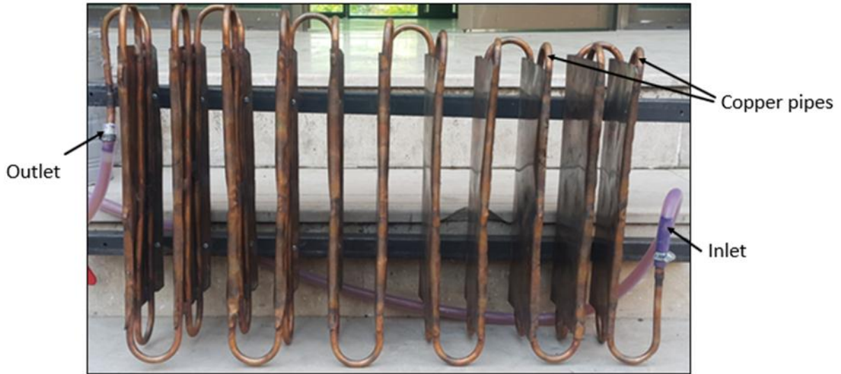
Figure 3.6 Arrangement of copper pipes inside container
