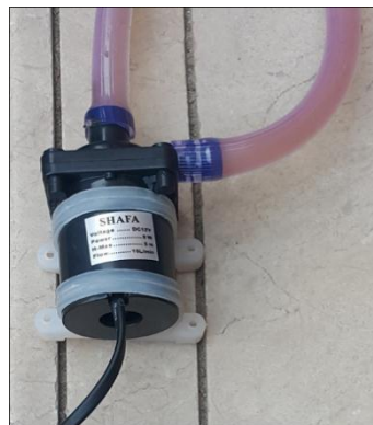
Figure 3.11 DC pump used to circulate water
