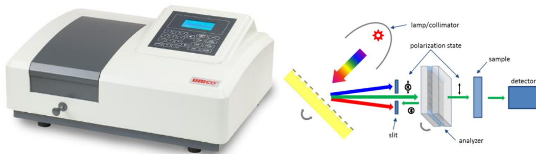
Figure 3.2: UV spectrophotometer and its working principle.
