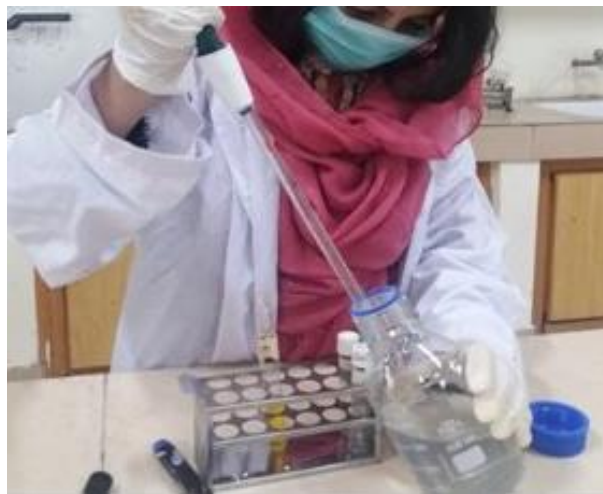
Picture 16 Preparing Samples for COD Test
