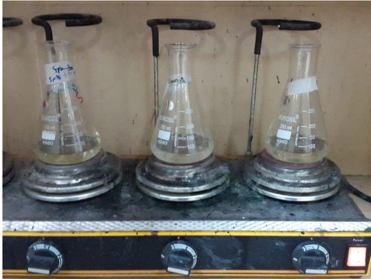
Picture 15 Sample Digestion for TP. Make: Valencia Scientifica. Model: ARE
