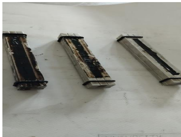
Figure 4-1:BBR molds filled with Bitumen Binder
