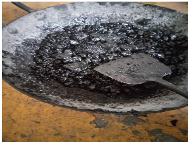
Figure 3-17: Prepared Asphalt Mixture
