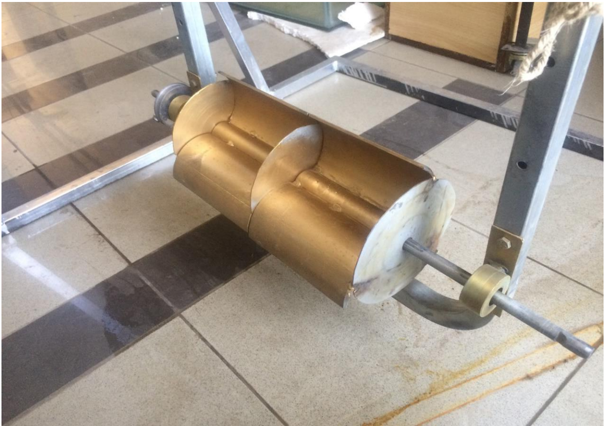
Figure 4. Double stage savonius rotor with three blades each
