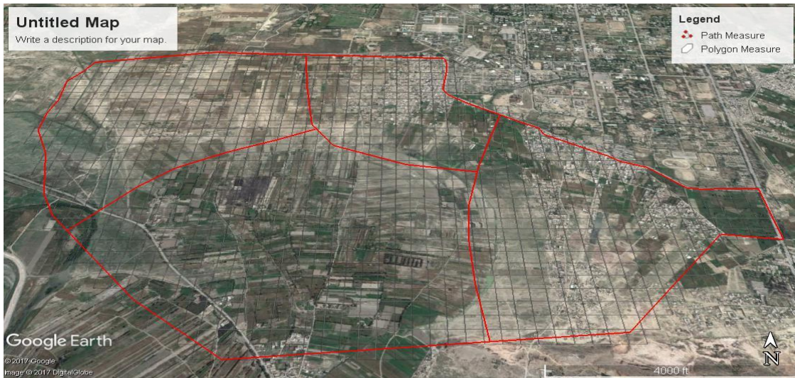
Figure 3.5: Template grid of size 100m sq. incorporated to Google Earth
