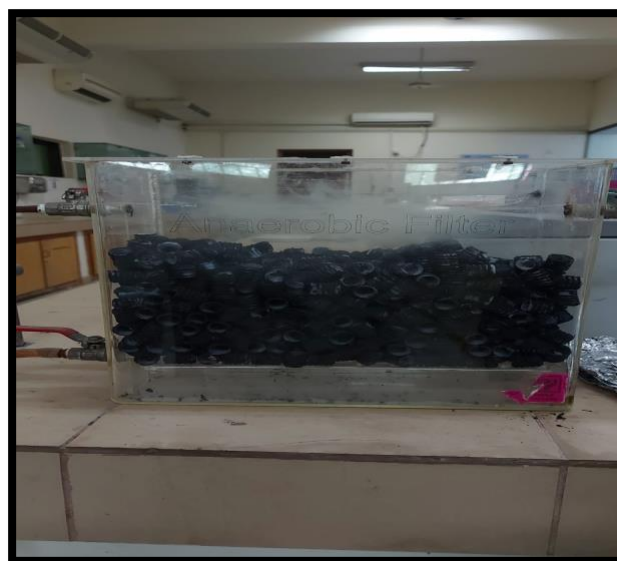
Figure 14: AF filled with Hybrid Media
