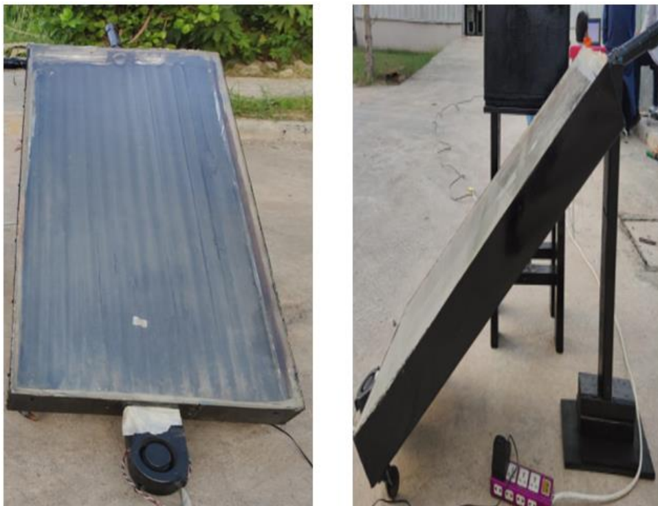
Figure 3-3. Front and side of solar air heater
