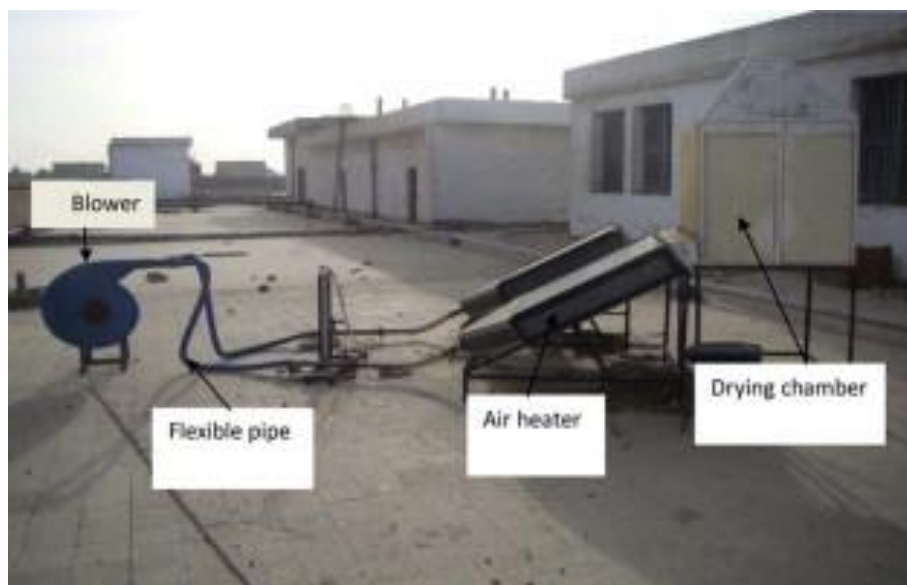
Figure 2-2. Indirect forced convection solar dryer [12]
