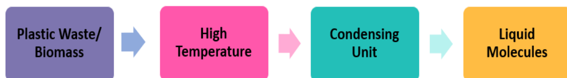
Figure 2.1 Steps in pyrolysis process
