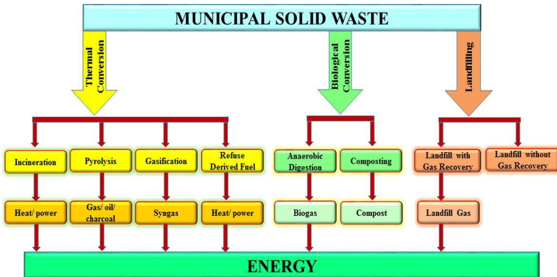
Figure 2.1 Flow diagram of different technologies for municipal solid waste treatment
