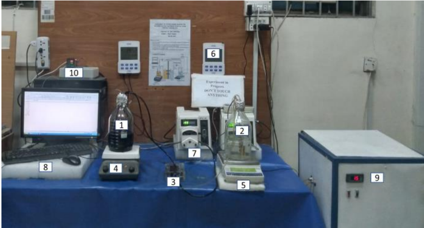
Figure 3.2: Batch Mode FO Setup(1) Feed Solution Tank (2) Draw Solution Tank (3) Membrane Module(47cm 2 ) (4) Hot Plate Stirrer (5) Weighing Balance (6) Conductivity Meter (7) Peristaltic Pump (8) Data Logger (9) Water Chiller (10) Temperature Controller
