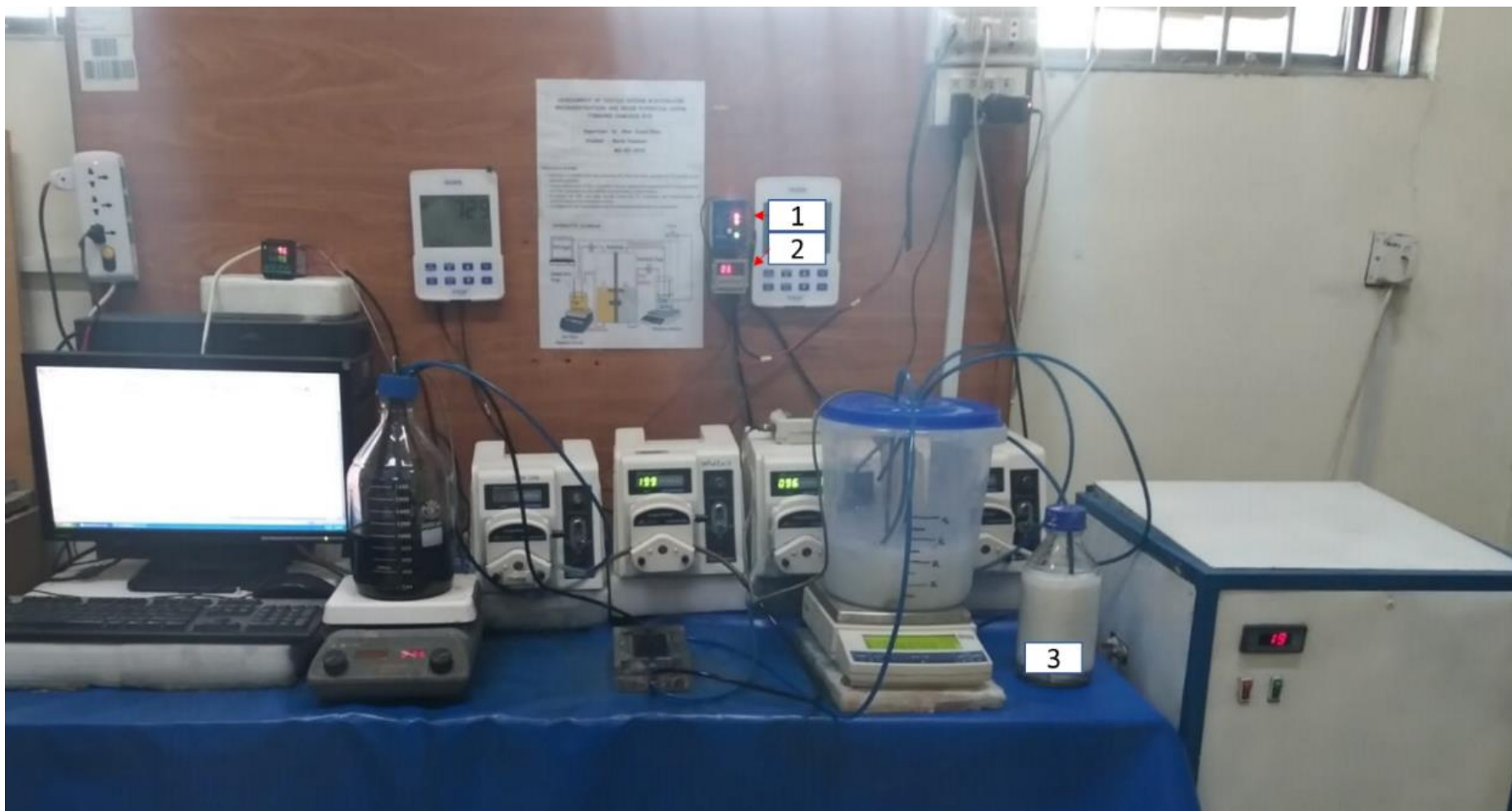
Figure 3.3: Semi-continuous FO setup (1) level sensor (2) time relay (3) concentrated DS (2M SDS) tank.
