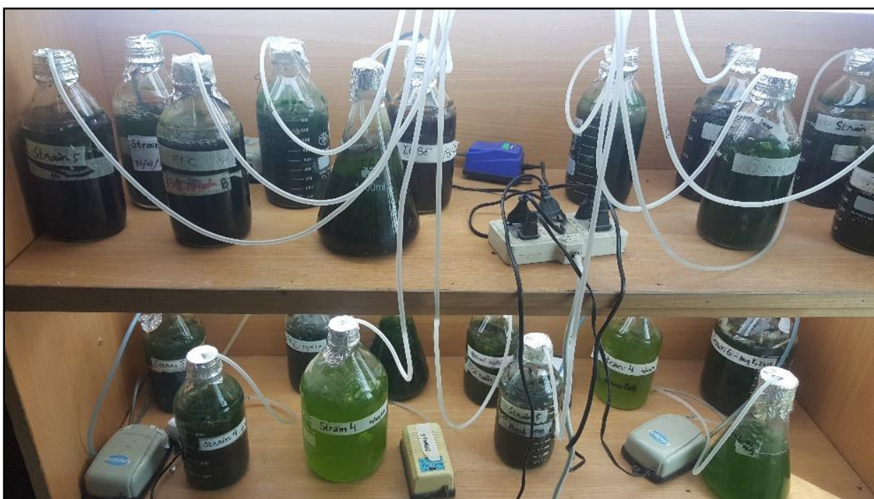
Figure 3.1: Algae growth culture setup at 25^{\circ}\text{C} , white florescent lamp at 10\mu\text{mol photons m}^{-2}\text{s}^{-1} with a 24hour light cycle
