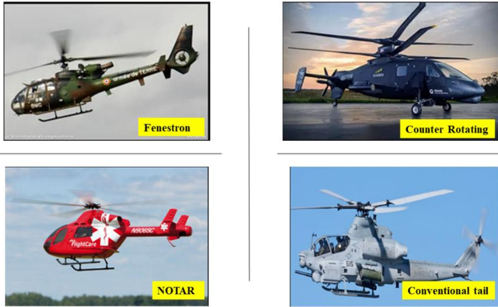
Figure 3-4: Four types of Rotorcraft configurations.
