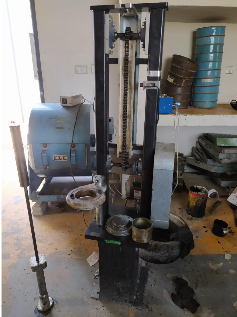
Figure 3.9 Marshall Compaction Machine
