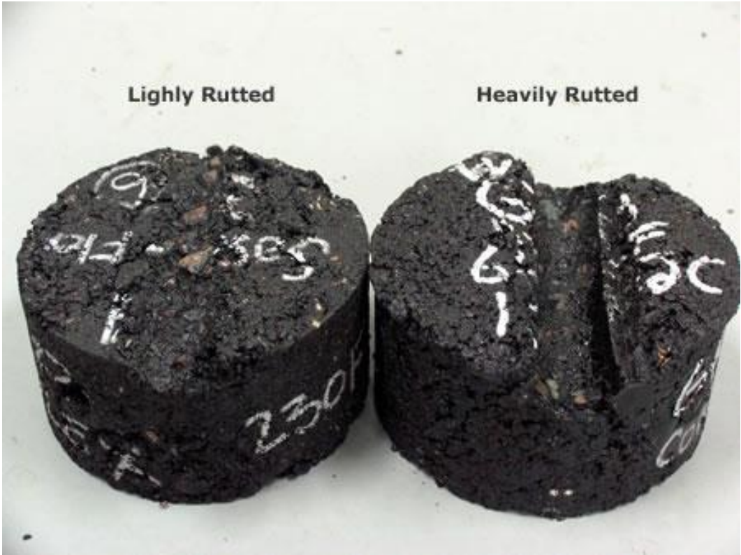
Figure 3.16 Rutting comparison of two specimens
