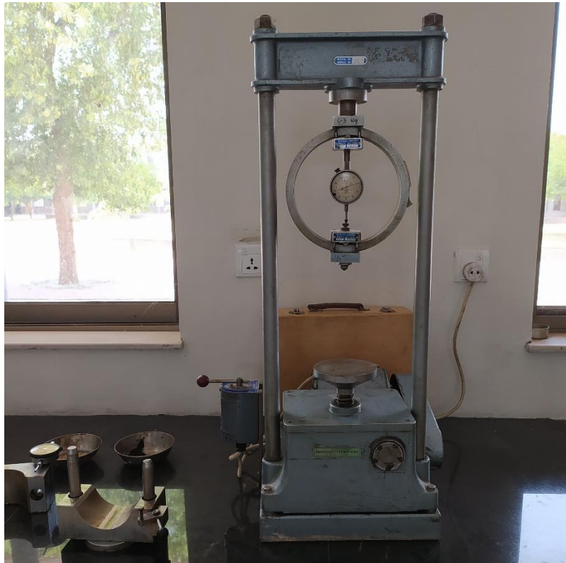
Figure 3.10 Flow and Stability Test Apparatus
