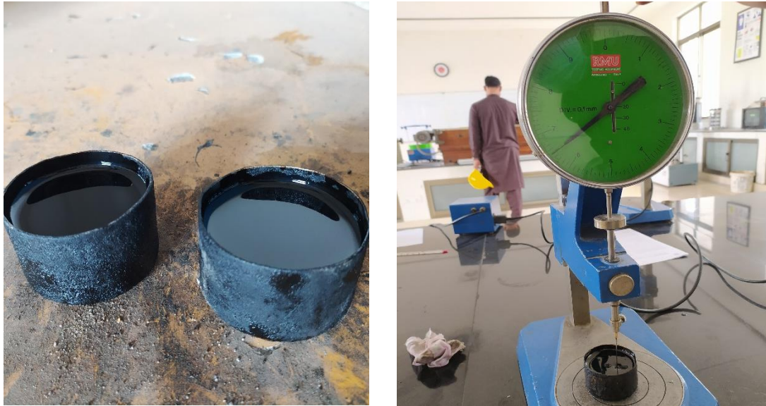
Figure 3.6 Penetration Test Apparatus
