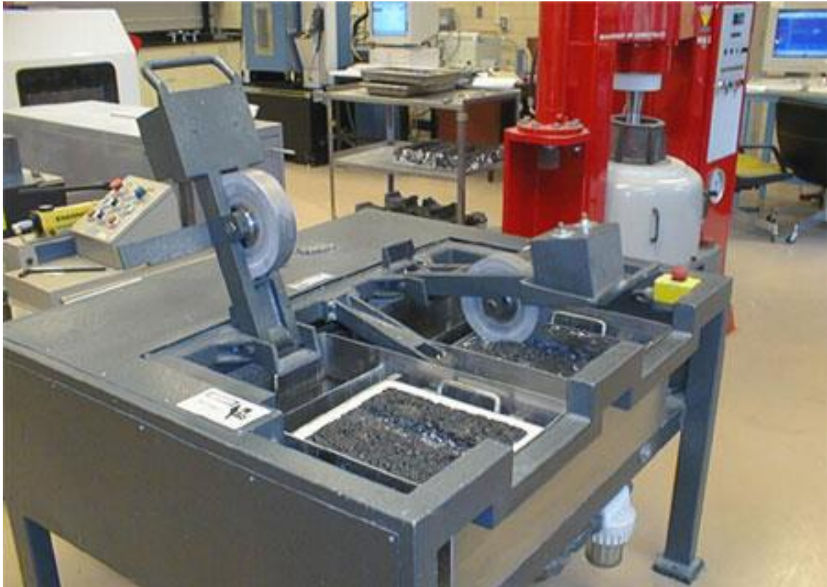
Figure 3.13 Hamburg Wheel Tracker Test Apparatus
