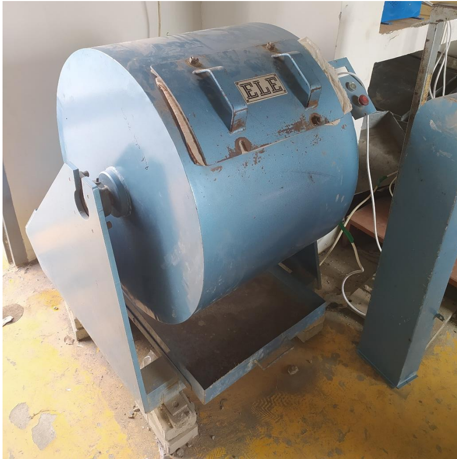
Figure 3.3 LA Abrasion Test Apparatus
