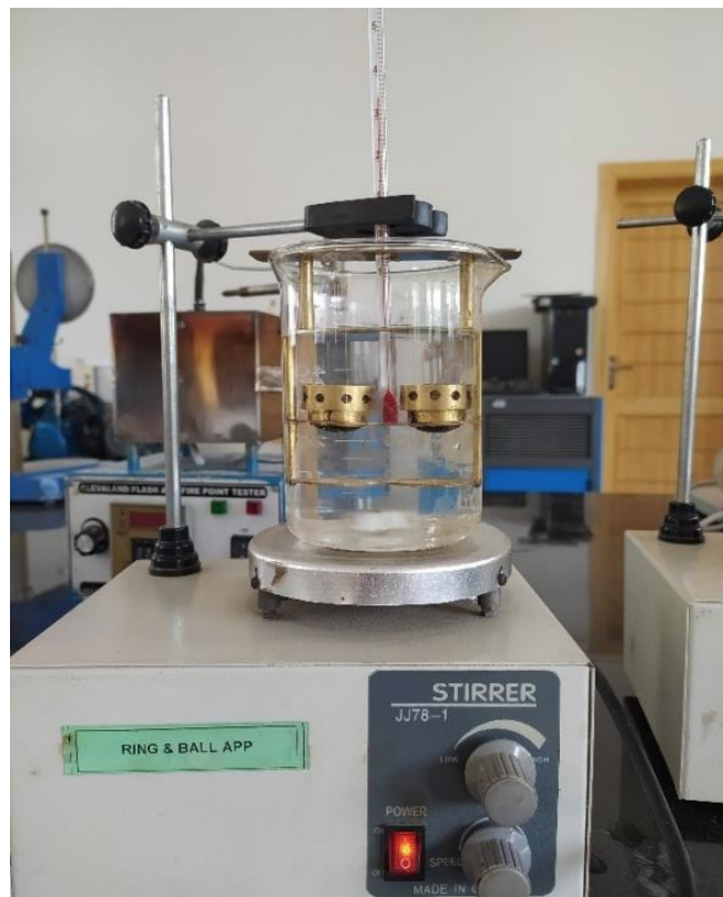
Figure 3.8 Ring and Ball Apparatus
