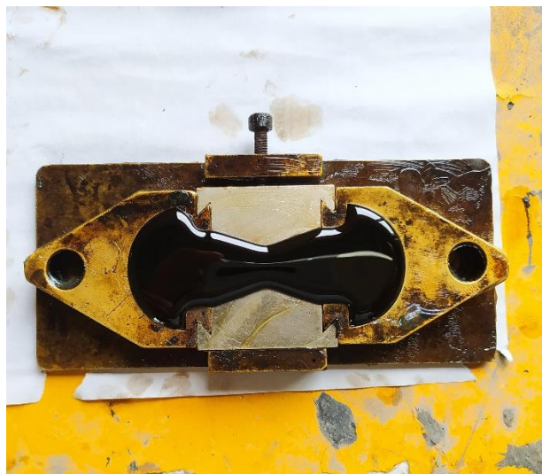
Figure 3.7 Specimen for Ductility test
