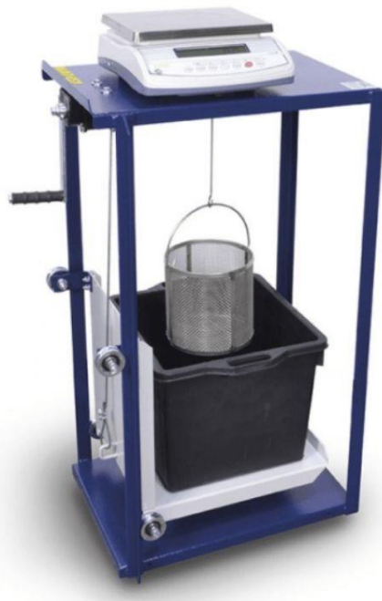
Figure 3.4 Apparatus for Specific Gravity of Coarse Aggregates
