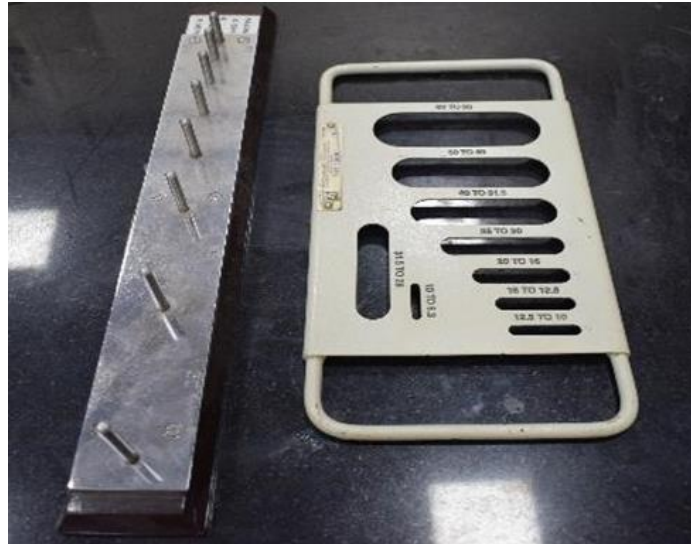
Figure 3.5 Flakiness and Elongation Index Test Apparatus
