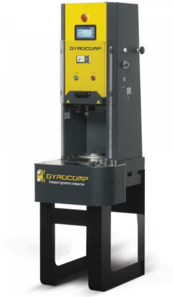
Figure 3.17 Gyratory compactor used for specimen preparation
