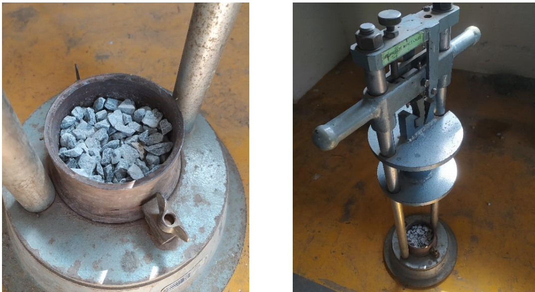
Figure 3.2 Aggregate Impact Value Test Apparatus
