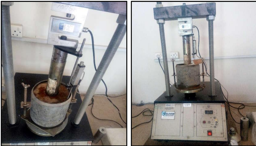
Figure; 3-8 (a,b) CBR Testing
