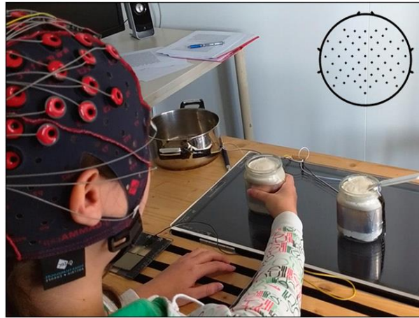
Figure 3-1 Experimental Setup of Gel-Based EEG data recording system [66].
