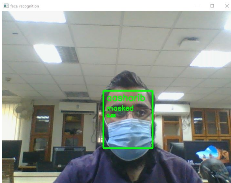
Figure 3.13: Face Recognition portal showing the name of the recognized entity along with mask status and cosine similarity score.
