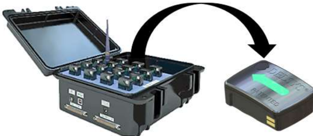
Figure 3.3: Trigno sensors Left- Base station Right- sensor
