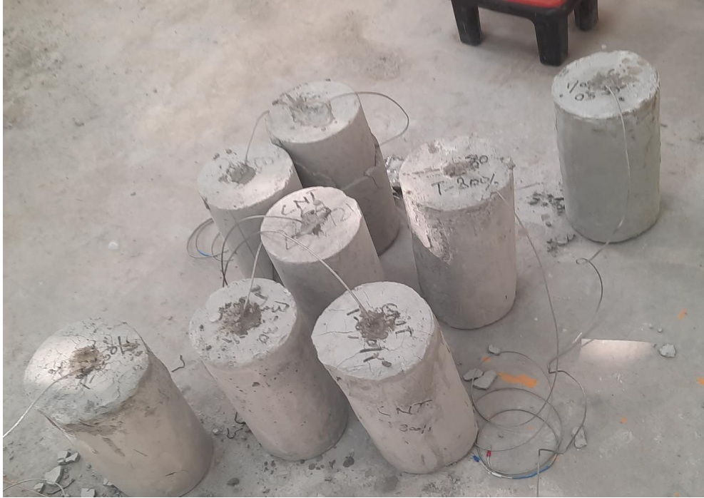
Figure 3: Thermocouple installed in Bentonite coated samples
