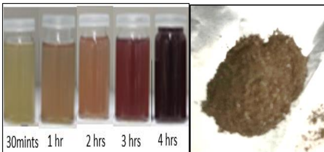
Figure 4.1: The color change represents the preliminary confirmation of silver nanoparticles. Purified AgNPs after drying are shown in the right panel
