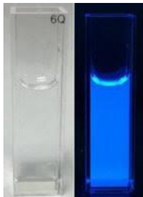
Image 4: Graphene quantum dots in visible light (L) and under UV light (R).
