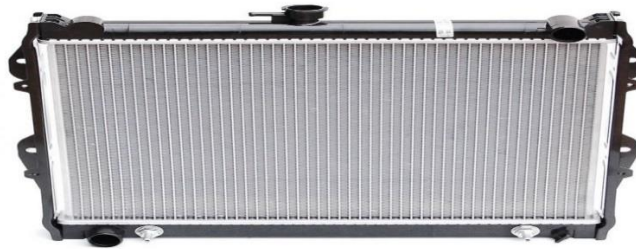
Figure 1.4 Gilled tube radiator [2]
