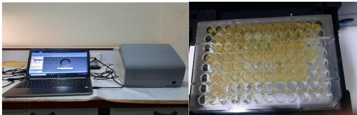
Figure 10: Microplate Reader in working and 96 well Flat Bottom Plate with Samples
