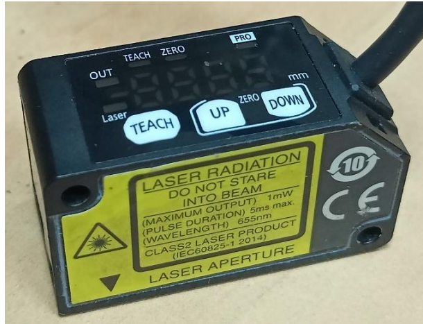
Figure 30 Panasonic HGC 1400 Laser Distance Sensor
