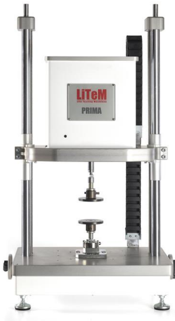
Figure 2 LiTeM Prima PN Fatigue Testing Machine
