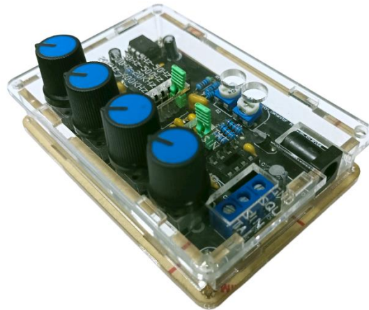
Figure 26 ICL 8038 Signal Generator
