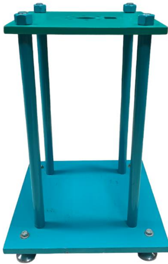
Figure 17 Base Structure for Fatigue Testing Machine
