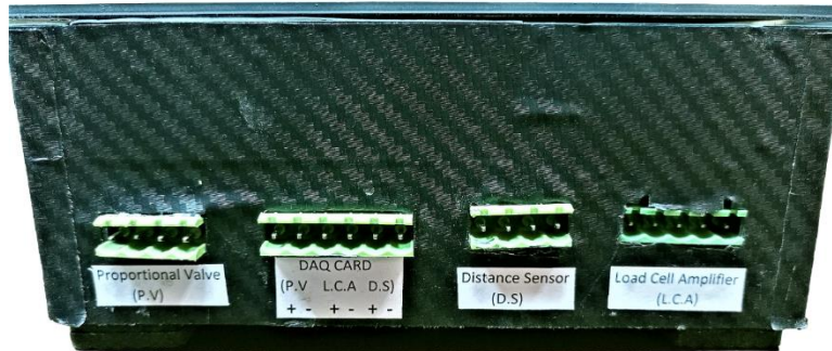
Figure 34 D.B Box Terminals
