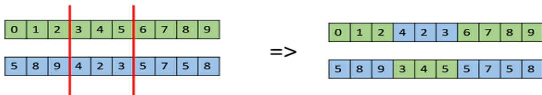
Figure 12: Double point crossover
