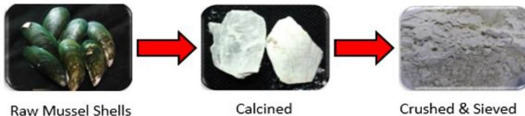
Figure 3-1: Calcination of Raw Mussel Shells.
