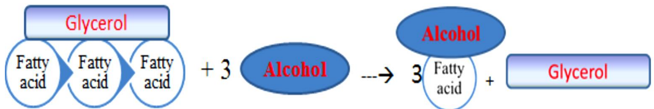
Figure 2-1: Chemical reaction mechanism of biodiesel production.
