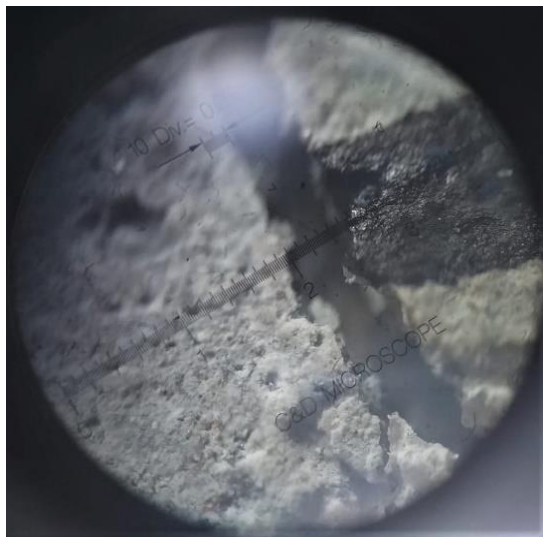
Fig. 4.19 (a) Control formulation crack day 1
