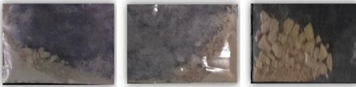
Figure 4 2 Precipitated calcite left to right: Calcium hydroxide (1420 mg), Calcium gluconate (460 mg), Calcium formate (260 mg)
