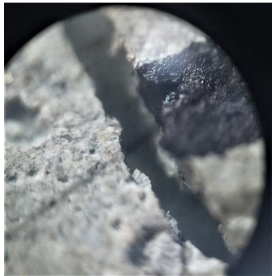
Fig. 4.19 (b) Control formulation crack day 7
