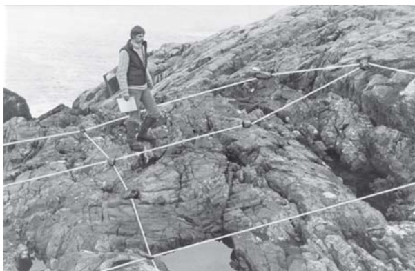
Figure 4.15 A 4 m cord mesh, used as a grid to aid sketch mapping, laid over an exposure at Badcall, NW Scotland (see Figure 4.16).
