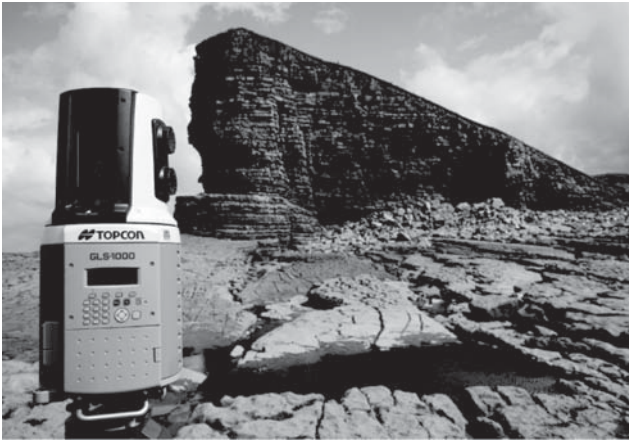
Figure 5.5 Terrestrial laser scanner being used by Terradat UK Ltd to make 3D scans of the geological cliff section at Nash Point, South Wales. Repeated scans are taken at regular time intervals and compared, to quantify rates of cliff erosion. Photo: Nick Russill, Terradat Ltd. Permission obtained from Terradat, UK.
