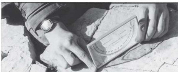
Figure 6.2 Using a 'Dr Dollar'-type clinometer to measure dip.
