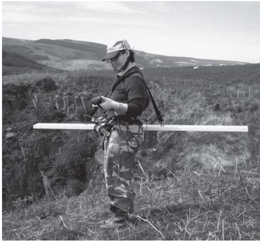
Figure 4.11 GEM-2 electromagnetic instrument coupled with a dGPS positioning system being used to help map faulted geological boundaries in the Rhondda Valley, South Wales.
