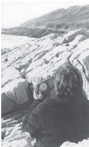
Figure 6.7 Measuring the dip of an uneven surface by Method 3 (see text).
