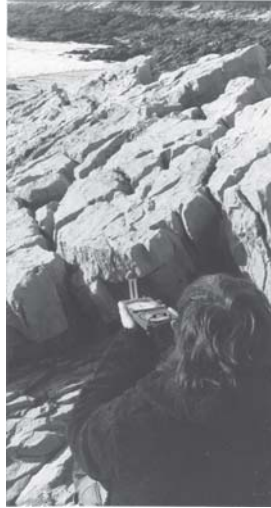
Figure 6.6 Measuring the strike of an uneven surface with a prismatic compass (Method 3; see text).
