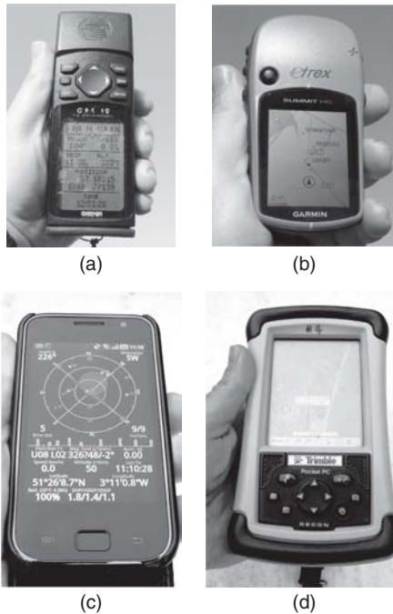
Figure 2.12 Some of the wide variety of hand-held GPS systems available on the market. (a) Basic rugged 12-channel Garmin GPS, which only provides locational coordinates but can be used with pocket PC (d). (b) Garmin GPS unit with ability to plot location onto a simple on-screen base map. (c) Mobile phone with GPS app installed. (d) Field-rugged Trimble pocket PC, which can take input from a GPS via cable or Bluetooth connection. A georeferenced air photo is shown on the screen. The software installed on the PC has the ability to log positional information along with field notes. Data can then be later automatically integrated into GIS software applications.
