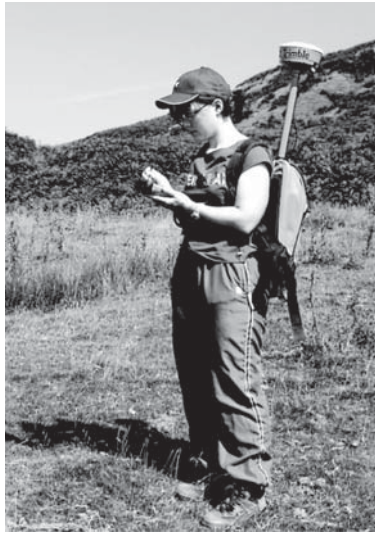
Figure 5.12 Adapted Trimble marine dGPS system being used for landslide mapping in South Wales. Note marine dGPS antenna housed in rucksack.
