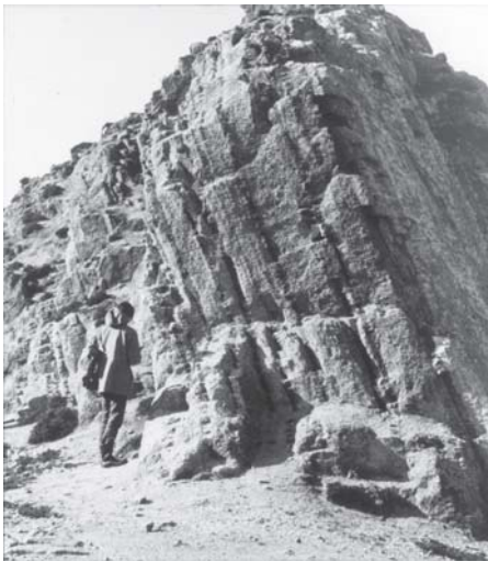
Figure 6.5 An ideal exposure for the end-on measurement of dip.
