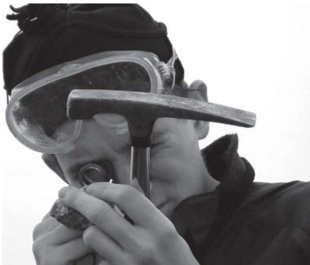
Figure 2.8 The hand lens is an essential tool for close-up study of rocks in the field.
