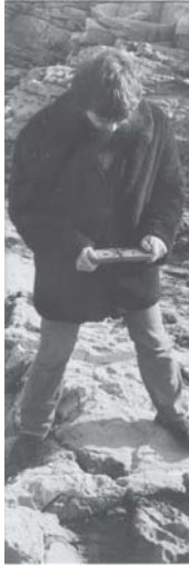
Figure 6.4 Measuring the strike of a veinlet on a rough horizontal surface by Method 2 (see text).
