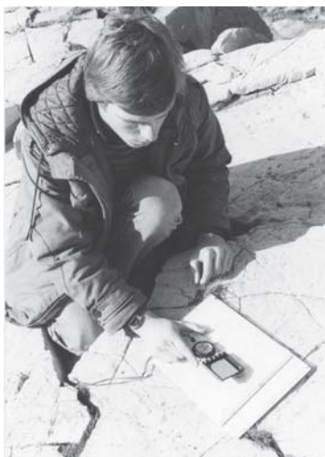
Figure 6.1 Measuring the strike by the contact method.
