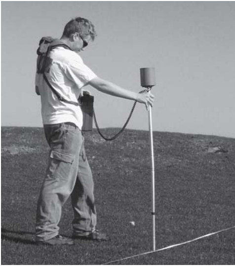
Figure 4.10 Proton magnetometer survey being carried out to detect and map a buried gabbroic dyke at Rhoscolyn, Anglesey, North Wales.
