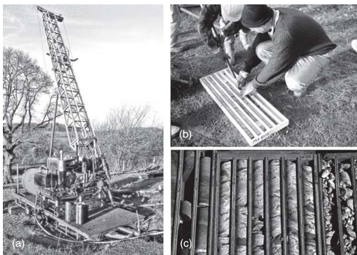
Figure 4.9 (a) Wireline, waterflush, rotary, diamond drilling exploration at Dolaucothi gold mine, Mid-Wales. (b) Cores retrieved from drilling. (c) Cores sequentially stored in core boxes and indexed against depth.
