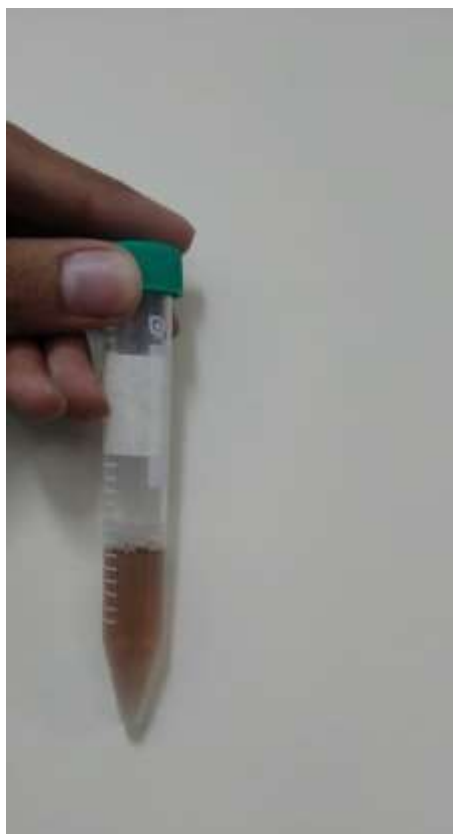
Figure 1 Figure depicting the colour change of the seed solution to dull-brown proving the formation of gold seeds in the process of synthesis of gold nanorods
