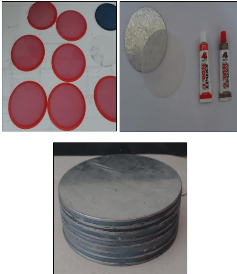
Figure 9: (a) Molding of silicone rubber layers in 3D printed molds (b) Steel and rubber layers along with the epoxy used (c) Prepared laminated Rubber Bearing
