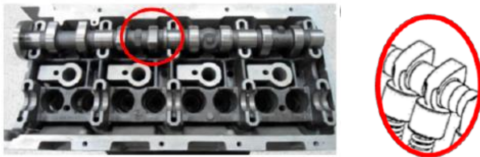
Figure 1. Test rig with the direct acting valve
