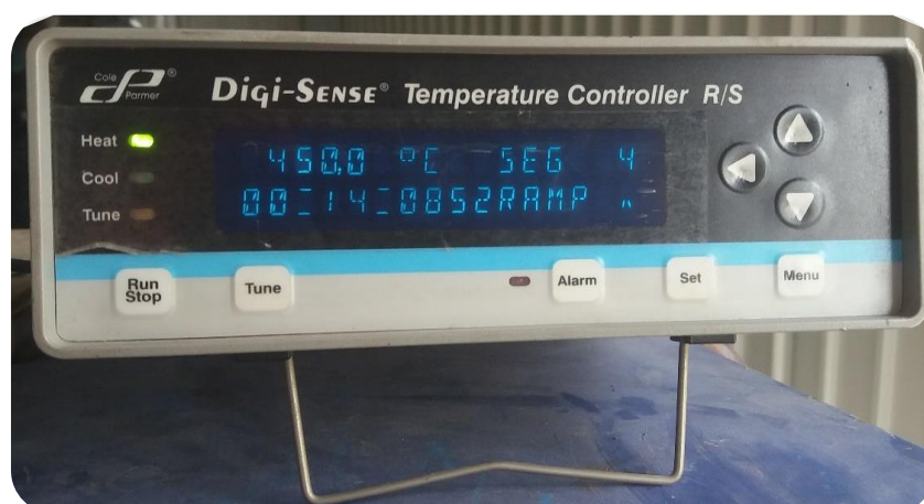
Fig. 3-5: Temperature controller of pyrolysis unit
