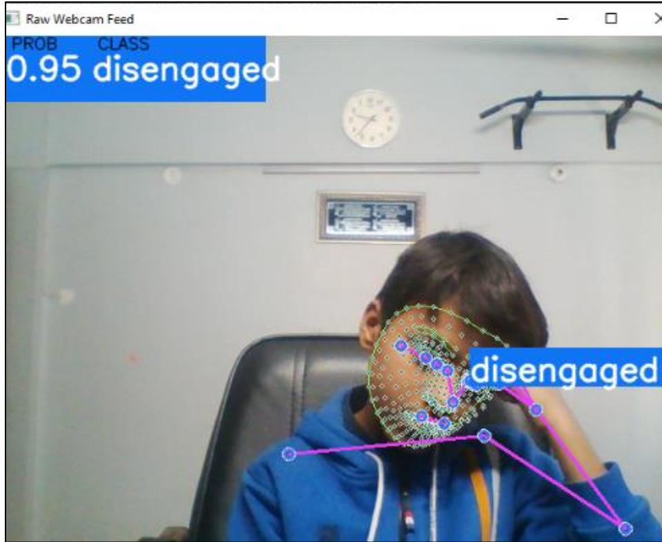
Figure 3.6: Realtime disengagement example of pose estimation via googles media pipe.
