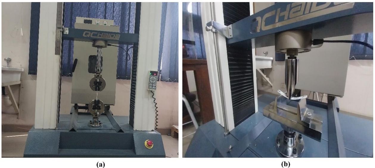
Figure 13. Haida UTM set-up: (a) Tensile set-up, (b) Flexural set-up
