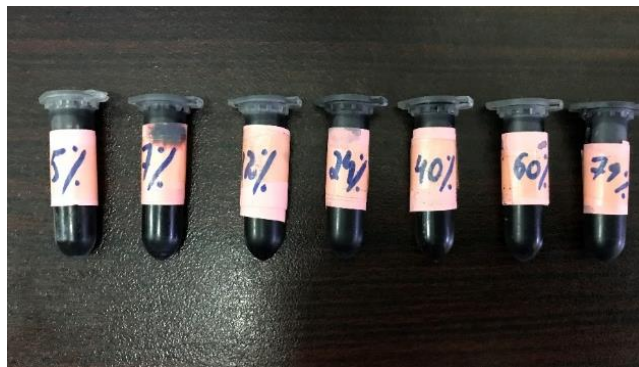
Figure 15: Seven Glycerin Solutions of Different Viscosities
