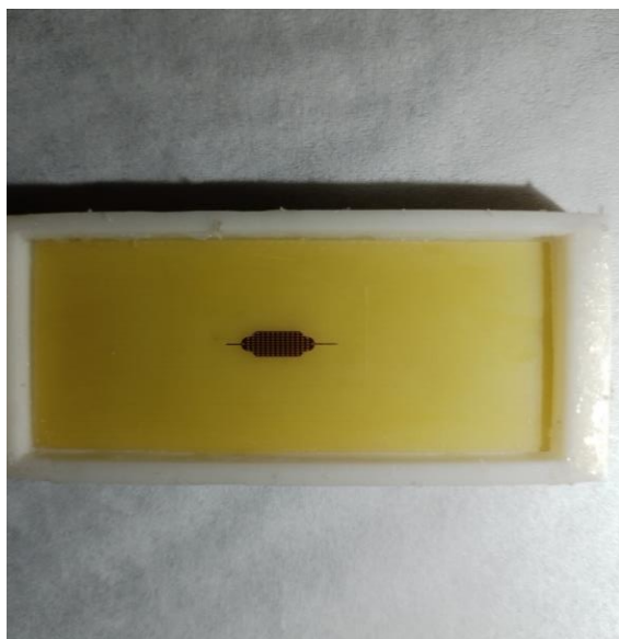
Figure 12: PCB Capillary Micropump in Silicon Mold
