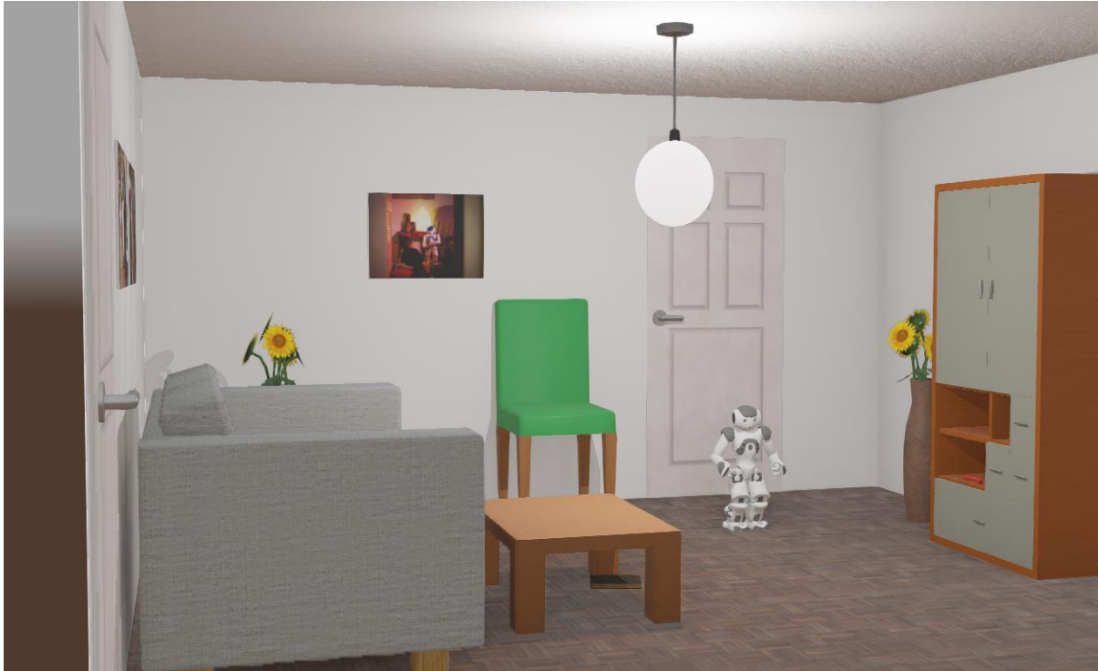
Figure 3.4: Virtual Reality platform for investigating HRI. The virtual robot in the framework is similar in appearance and capabilities to the Nao robot by Softbank Robotics
