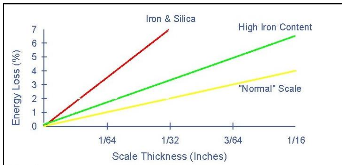
Figure 1.2.2: Above Figure shows the graph of scale thickness vs Energy Loss % [8]
