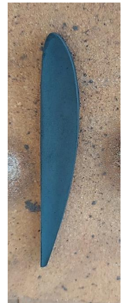
Figure 3.4: The final Cupric Oxide ceramic part resting on firebrick after sintering process.
