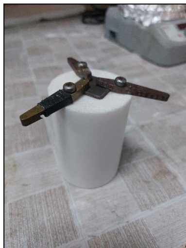
Figure 14, Sample attached to the EPD cell using screws.
