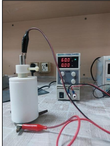
Figure 17, EPD cell connected to a DC supply with a voltage of 60.
