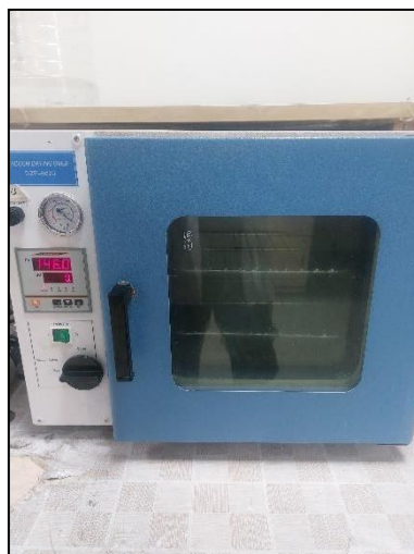
Figure 18, Drying oven set a temperature of 150 degrees.
