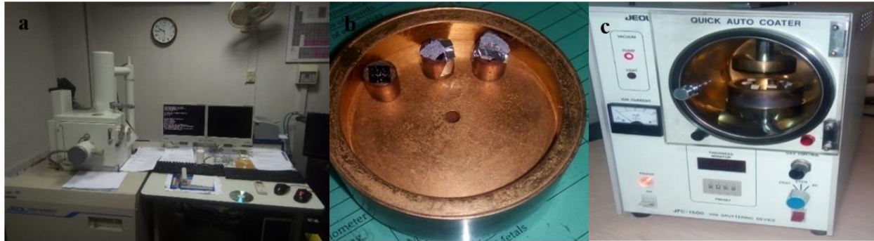
Figure 3.12. (a) Scanning electron micrograph apparatus (b) Samples (c) Gold plating of samples
