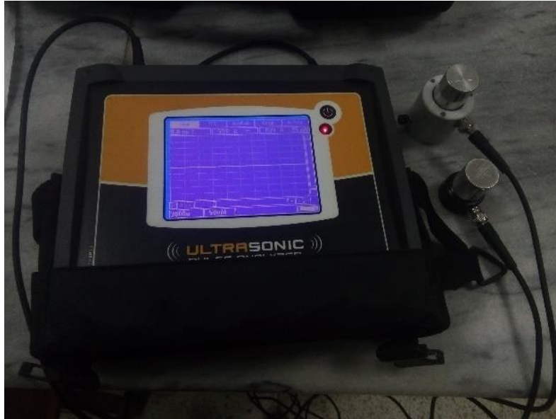
Figure 3.11. Ultra-sonic pulse velocity test apparatus.
