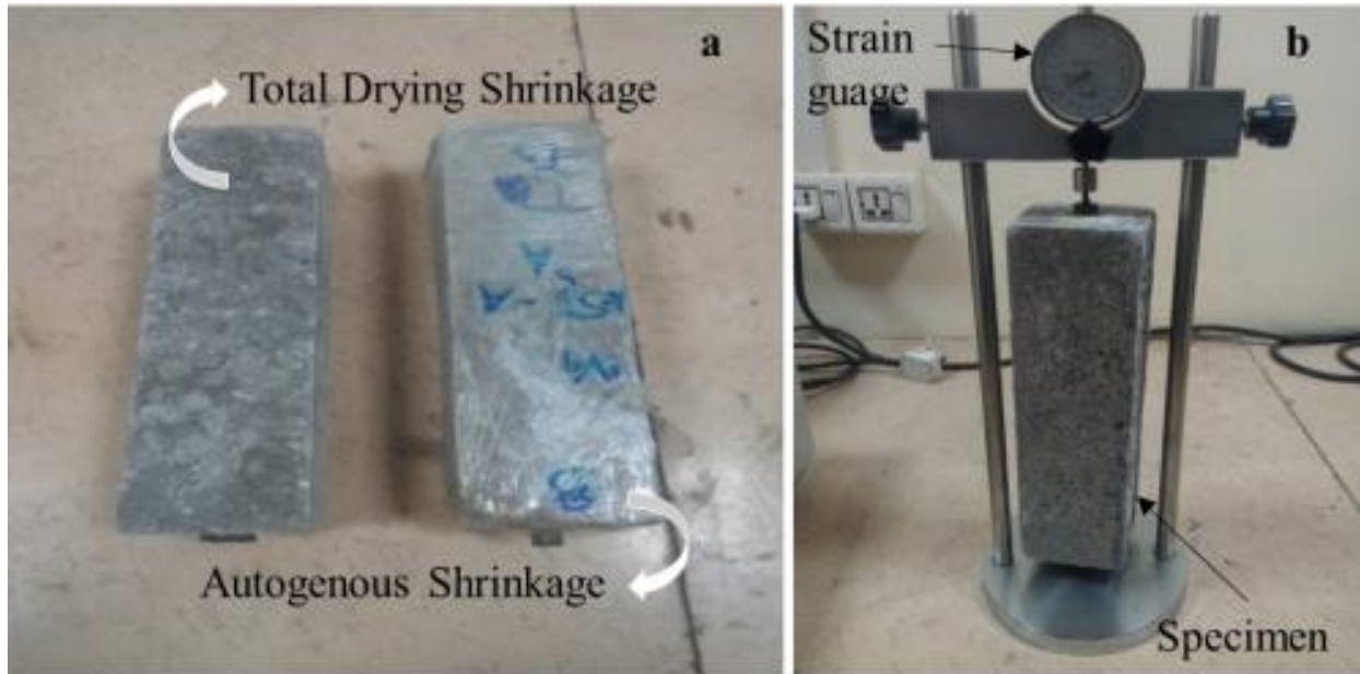
Figure 3.8. (a) Samples for autogenous and drying shrinkage (b) Shrinkage test apparatus.
