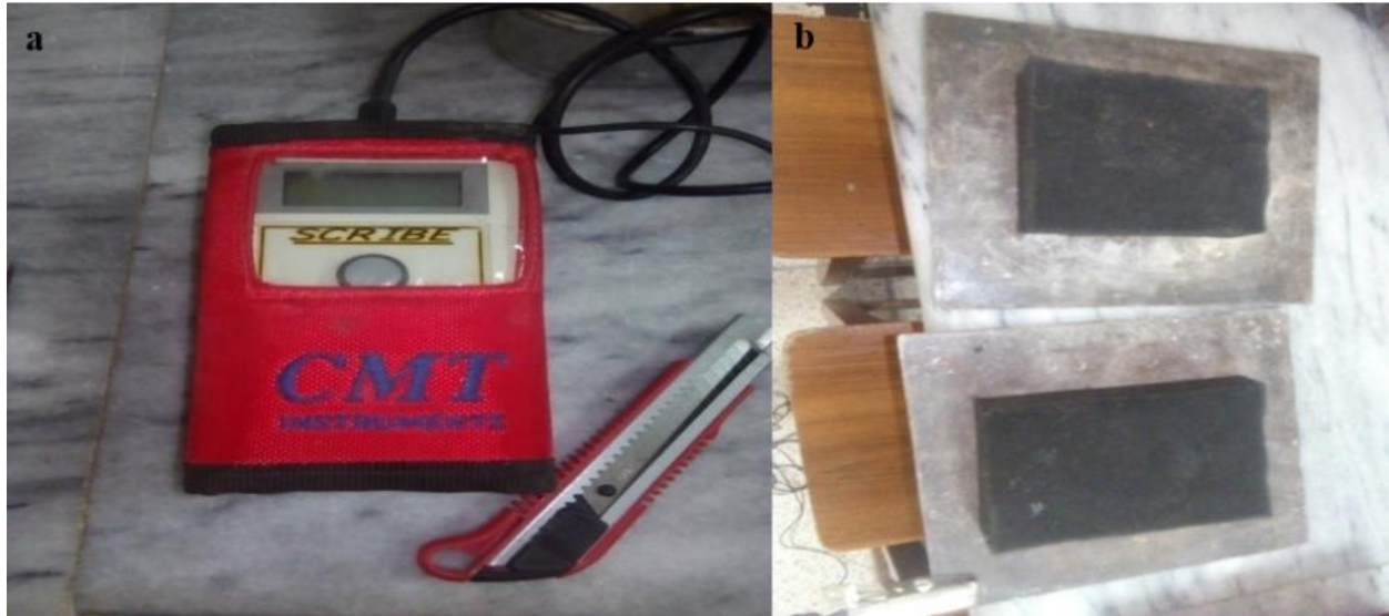
Figure 3.9. (a) Bulk resistivity test apparatus (b) Electrode plates
