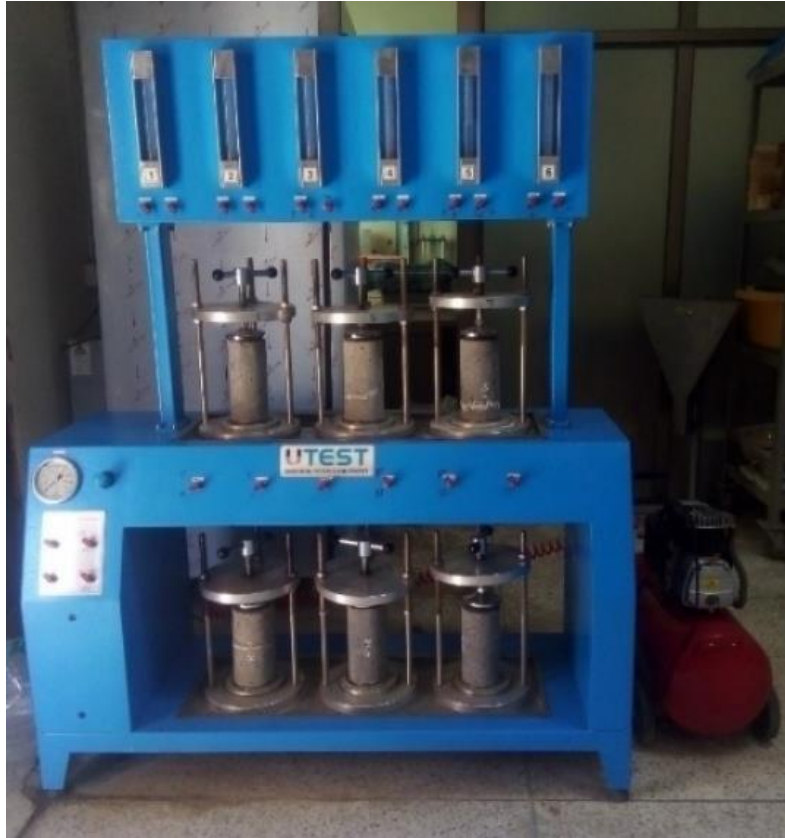
Figure 3.10. Permeability test apparatus.
