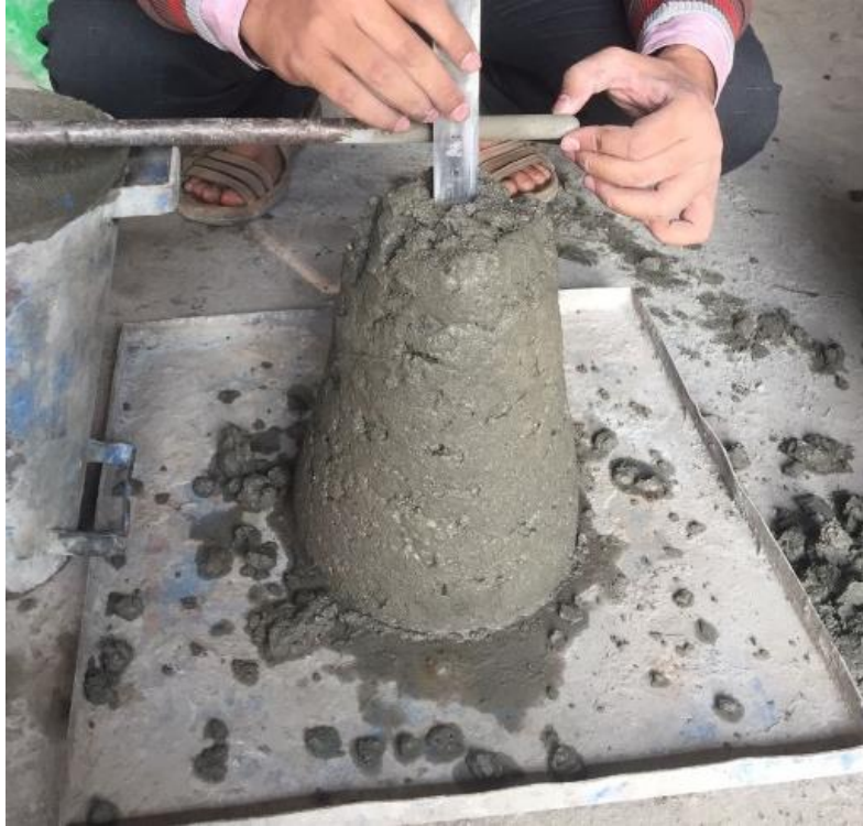
Figure 3.4. Workability test using slump cone apparatus.
