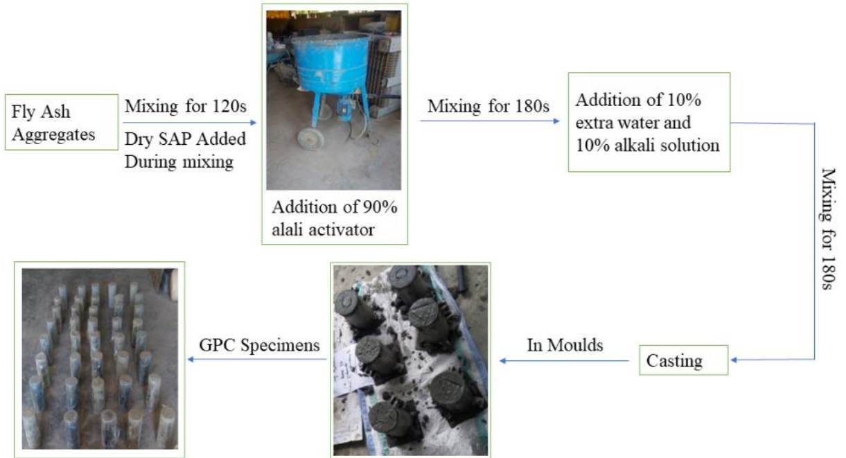
Figure 3.2 Mixing procedure for GPCs.
