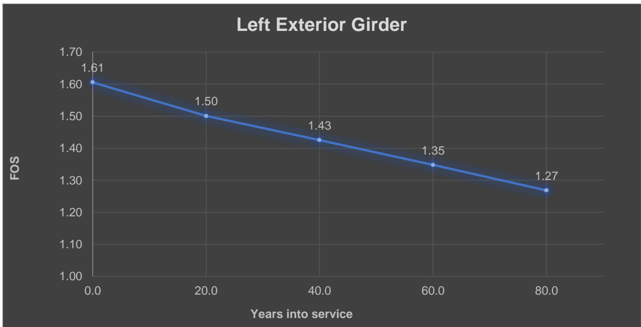
Figure 28 FOS Left Exterior Girder over 80 years.
