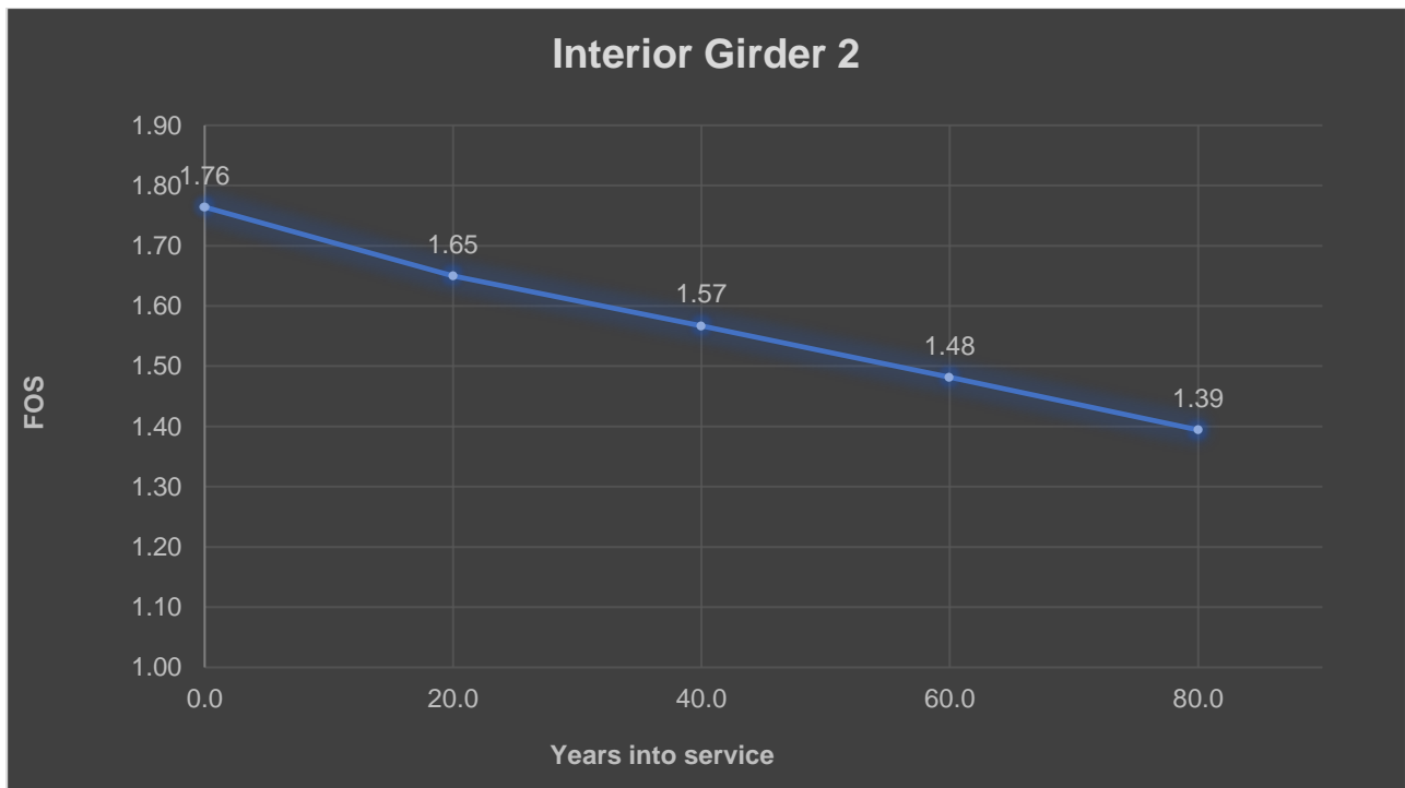
Figure 26 FOS Interior Girder 2 over 80 years
