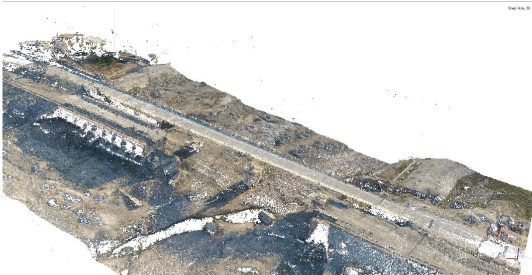
Figure 8 Step 1: Photogrammetric point cloud.
