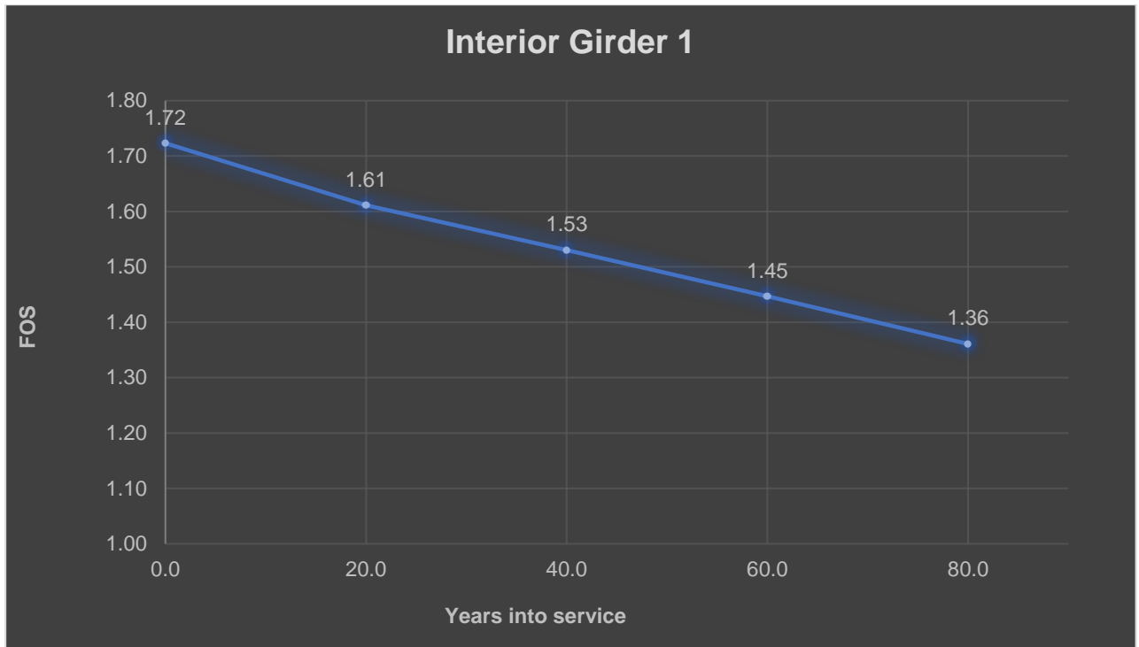
Figure 25 FOS Interior Girder 1 over 80 years
