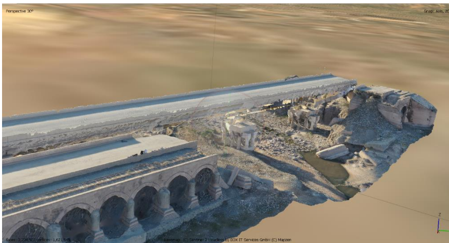
Figure 10 Step 3: Photogrammetric textured Model (AGI Meta shape)
