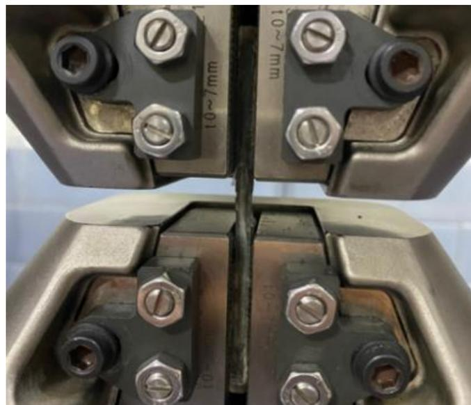
Fig 25: Composite Sample in UTM Jaws
