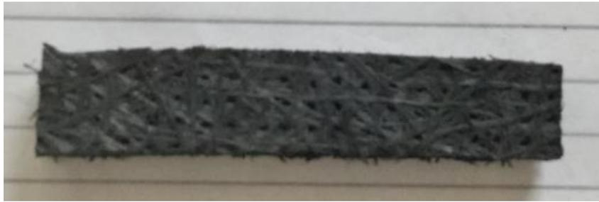
Fig 8: Sample After Pyrolysis
