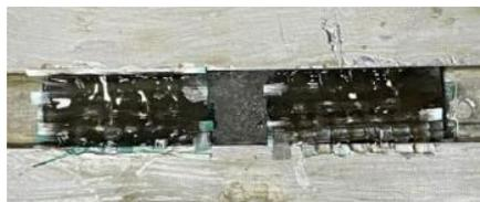
Fig 22: Tabs attached on Grip Section
