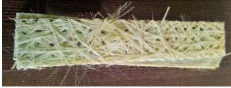
Fig 11: Thermally Treated Fibers
