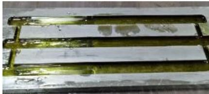
Fig 20: Mold with Fibers plus Resin
