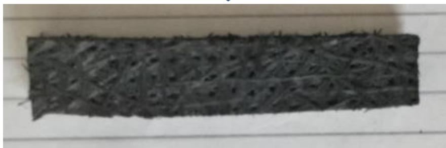
Fig 7: Carbonaceous Layer Present on Sample
