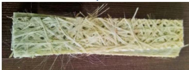
Fig 10: Sample after Post-Oxidation
