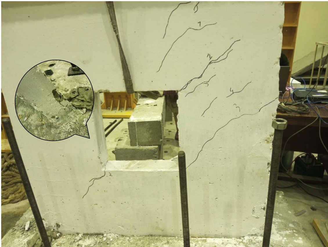
Figure 11 : Wall 1:1 Crack Pattern
