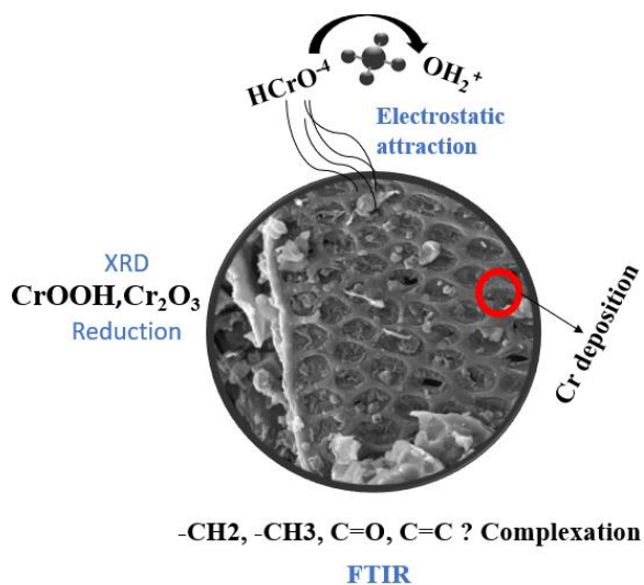
Figure 17. Cr (VI) removal mechanism
