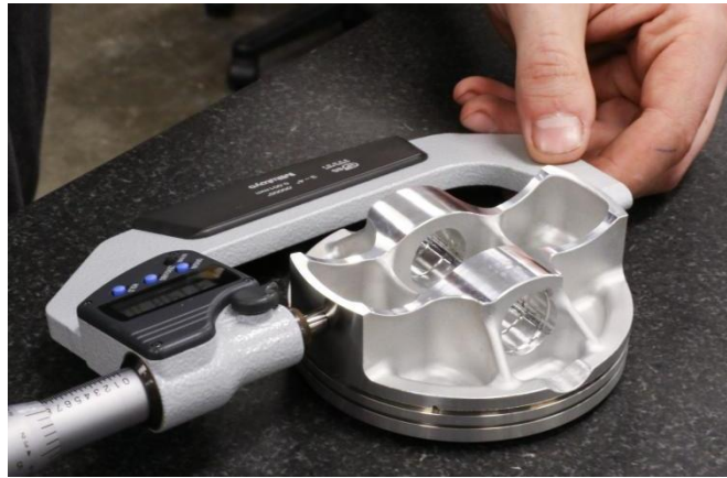
Figure 6: Ovality measurement through Micrometer
